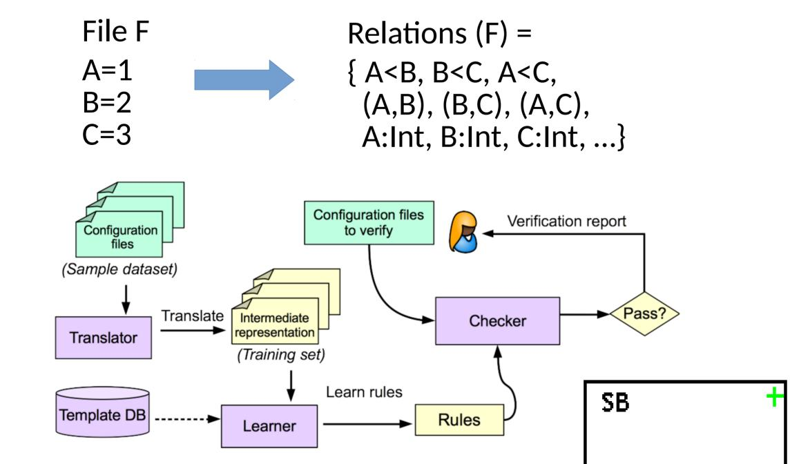
Status(F) = Pass  $\Rightarrow \forall r \in \text{Relations}$  (F),  $r \notin \text{Breaking}$ Status(F) = Err  $\Rightarrow \exists r \in \text{Relations (F)}, r \in \text{Breaking}$
